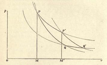
corresponding to an infinitesimal change of volume. We thus obtain (as in § 190) a number of narrow rectangles, the sum of whose areas is ultimately the curvilinear space MPP'M'. Similar constructions must be made for the expansion from P' to Q' and the contractions from Q' to Q and from Q to P.
